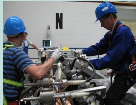
Clamping of the bus bars to the structure
