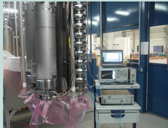
HOM tuning and cable connection
