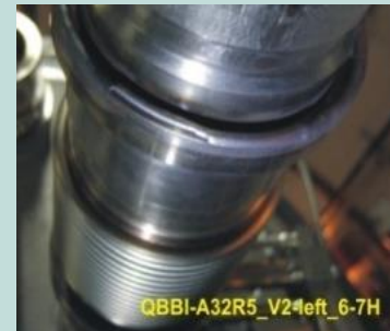
Non-conforming weld (left) and compensation bellow (right)
