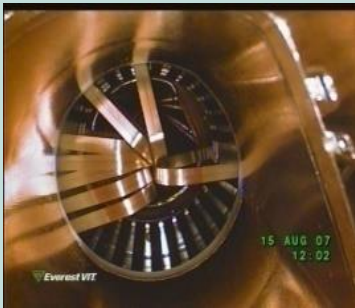
A plug-in module (PIM) damaged during a cool-down/warm-up thermal cycle of the magnets
