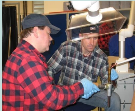
Tinning of the bus bar super conductors
