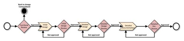
Input to the Procedure is a conducted PDR (Preliminary Design Review) of the parent system. Outputs are released BOMs (Bill Of Material), Descriptions and Specifications of a Part/System.
