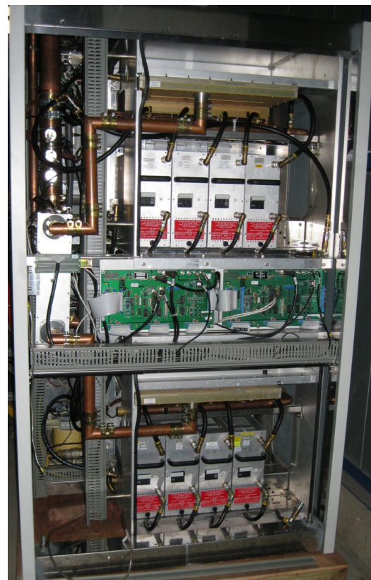
Thomson 10 kW Solid-state amp for testing HWR couplers at Argonne
