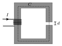
Consider the circuit in the figure. The grey part is iron and the white is air, or vacuum. The air gap d is small. We assume that the permeability of the iron is very large and that the leakage of magnetic flux is negligible. Ampère's law (10) gives
