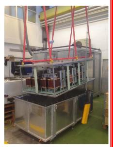
2. Preliminary testing of HV oil tank assembly at low voltage - 24<sup>th</sup> March 2016;
