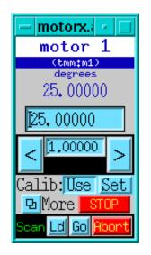
Available operations from this display; Make absolute or incremental moves. Define the current position. Stop the current move. without any controller specific information.
