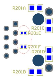
Settings of both solder bridges are shown below. To establish state closed a solder bridge (0 Ohm 0402 resistors) must be installed.
