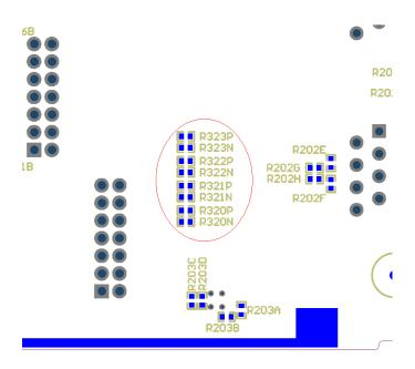
Routing table and settings of solder bridges are shown below. To establish connections to appropriate I/Os of Zone3 connector the corresponding solder bridges (0Ohm 0402 resistors) must be installed.
