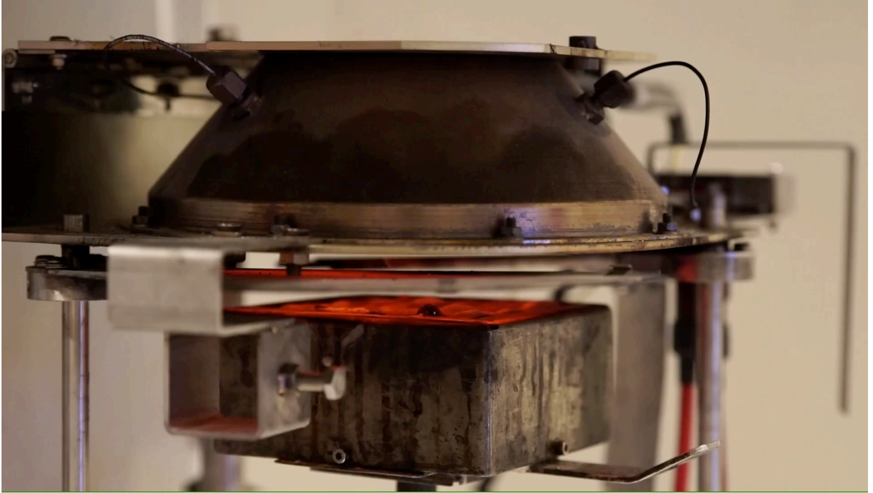
T. Hehnen and M. Plagge, Cone Calorimetry of CERN-specific cables at Lund University, June/July 2017
