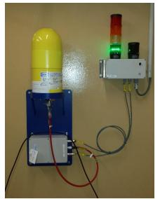
Ionizing chamber 150 nSv/h-0,15 Sv/h OK for Pulsed cycle
