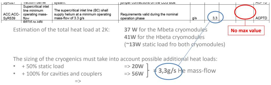
Sizing of the internal heat exchanger: **4,5g/s max for the M-ECCTD**.
