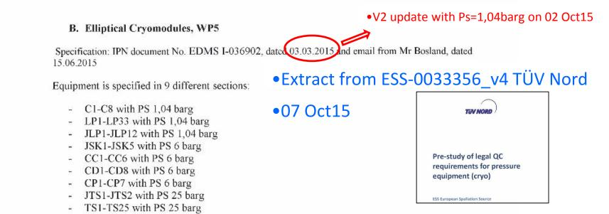
Classification according to figure 2 (pressure vessels) or figure 7 (piping) in PED, appendix 2, was checked. Due to small equipment (volume not above 49,9 litres and DN not above 960 mms for 1,04 barg, not above 8,33 litres and 200 mms for 6 barg and not above 2 litres and 40 mms for 25 barg) all pressure equipment is classified according to PED, article 3.3.
