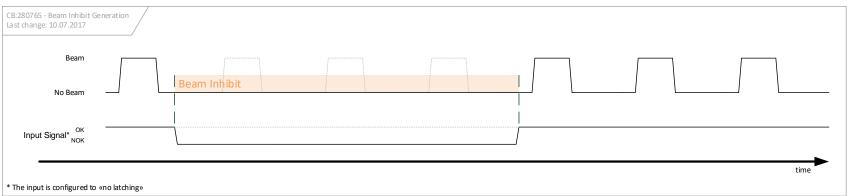
OK→NOK transition of input configured to «latch NOK» when there is no beam:
