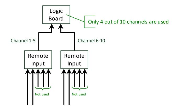
Arrange connection of signals to the FBIS such as to avoid unused inputs.
