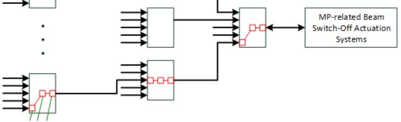
Implement the FBIS such as to maximize the number of inputs that can be processed in one single step in order to minimize tree depth.
