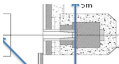
Fig. 20 beamstop layout for ERNIS imaging instrument under construction at JPARC [28]
