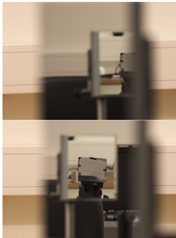
Figure 4: The top image is taken with the camera placed a few cm off the optical axis outside M4 by. The bottom image is taken after adjusting M4 to center the optical axis on the camera.
