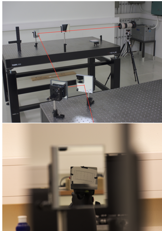
Figure 3: It is possible to find the optical axis on top of the PBIP by using a camera. The camera is not perfectly centered on the optical axis, as the camera is simply placed by hand on a tripod. The optical axis is where both M1 and M4 are centered on the image.
