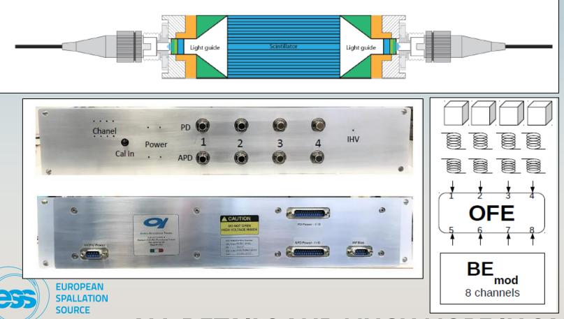
**Optical Front End** (**OFE**) prototype 8 channel IN 8 channel OUT 2 signal \ SCINT 4 SCINT \WS FO from WS to OFE Up to 150m Modified Back End (BE<sub>mod</sub>)
