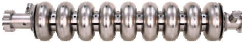
TESLA 9-cell 1.3GHz cavity
